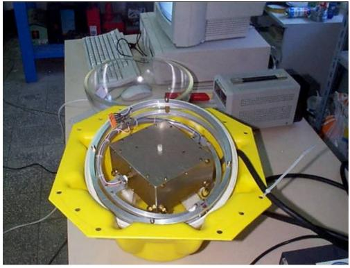
Figure 1. Gravimeter installed inside the bentos sphere by means of the gimbals suspension.
