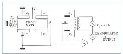
Figure-3 Simple scheme of the gravimeter read out system.
